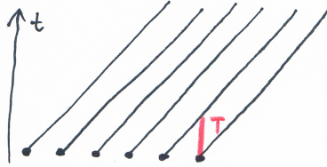
Figure 4: The electric current I relates to the time lapse T needed for an electron to take the position of its predecessor.
