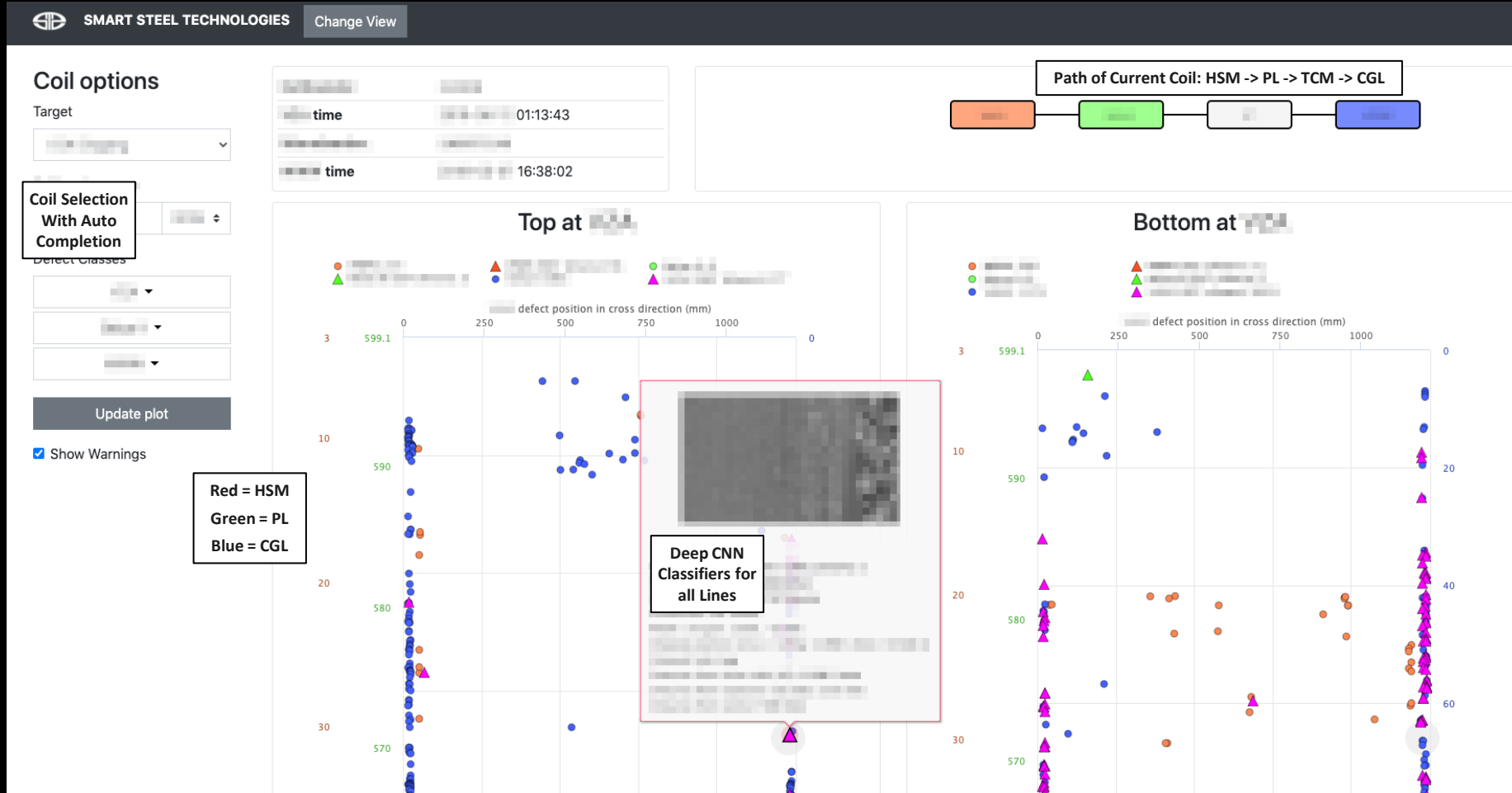
Matching of defect positions across all routes: HSM, PL, TCM, CGL, inspection lines
